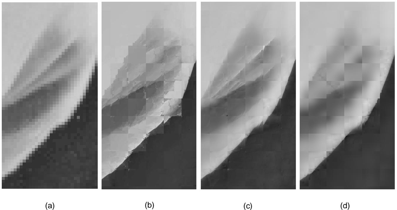
Figure 3. Zooming x16 (x256 pixels) in fractally encoded images with fixed 6x6 child blocks. (a) Original image. enlarged by pixel replication. (b) Zoomed fractal with DC basis and local searching. (c) Zoomed fractal with limited cosine basis and local searching. (d) Zoomed implicit fractal.
