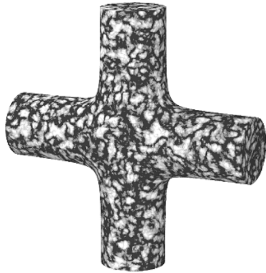
Figure 5. Blended union of two cylinders
